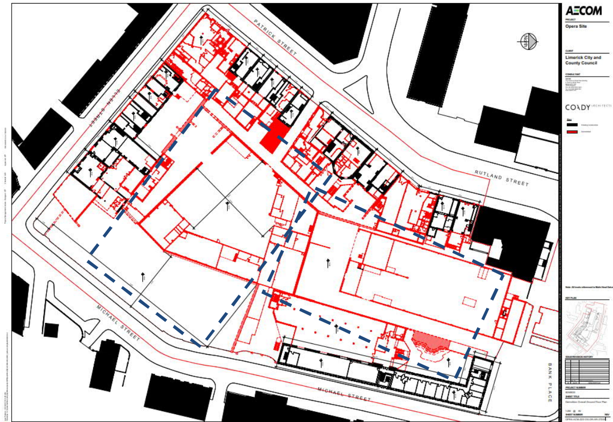
Figure 2 Existing Site Plan with proposed demolition in red, indicative areas for construction compounds in blue and building which will be subject to work in the enabling stage as black outlines.
